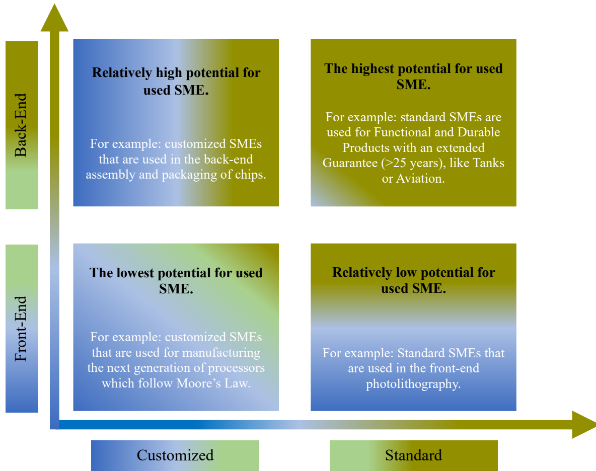
Figure 10: A 2x2 matrix focused on the equipment type and semiconductor process of the used semiconductor manufacturing equipment (SME)
